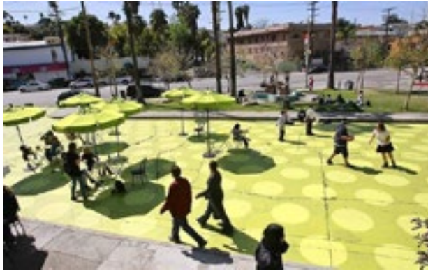
Street space converted into an interim plaza using low-cost materials (paint, tables and chairs, basketball hoop) in Los Angeles, CA Source: NACTO
